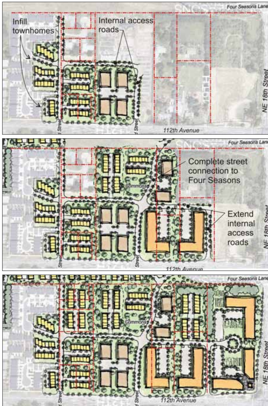
Figure 11. Illustrating how individual developments could be integrated over time with collaborative site planning. Example phases over twenty years.
