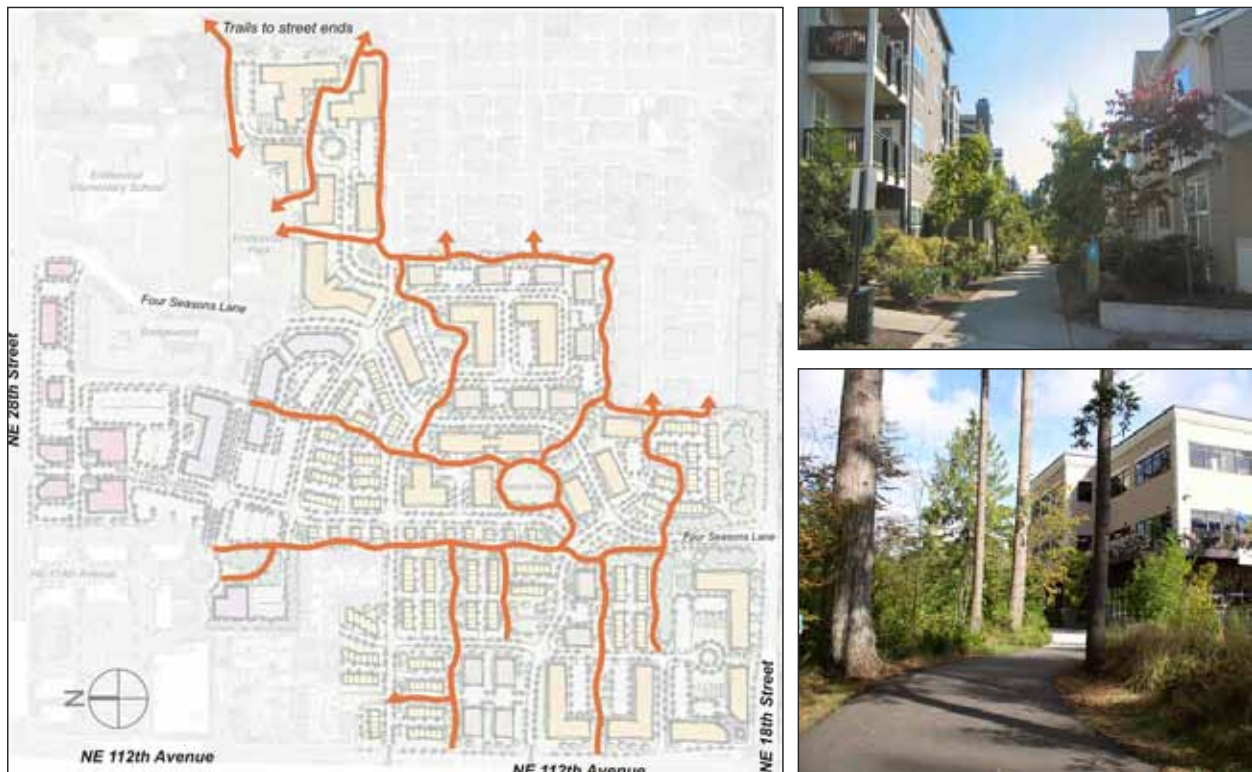
Figure 10. Illustrating the off-street trail network in the site plan example plus trail design and context examples (right)
