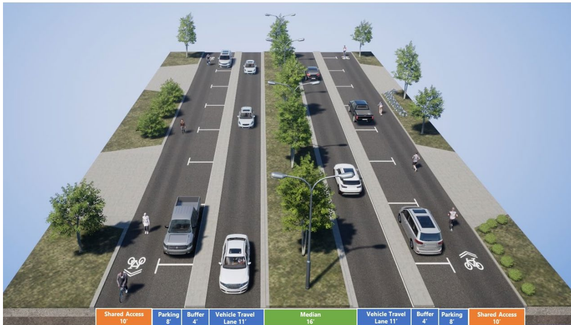
Figure 4. Design Option 3: Shared Mobility Lane/Residential Access
