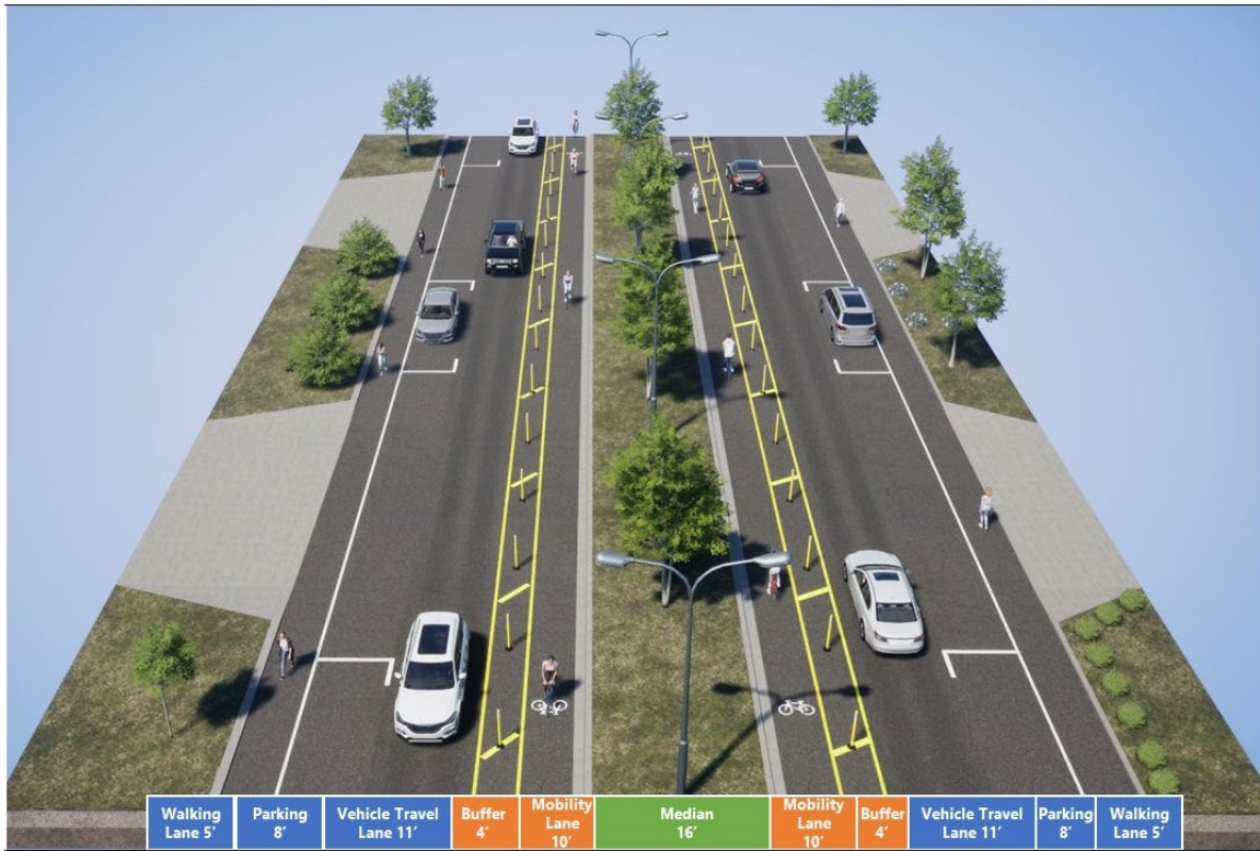
Figure 3. Design Option 2: Center Running Mobility Lane
