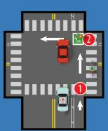
Two-stage left turn boxes are designed to give bicyclists a safe way to turn left through an intersection
