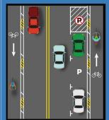
Parking-protected bike lanes include bike lanes by the curbs. with buffer areas on the driving lane sides. There is a parking lane between the bike lane buffer and the driving lane on one or more sides of the street.
