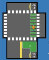
Bike lane extensions are designed to provide a visable area of travel through an intersection
