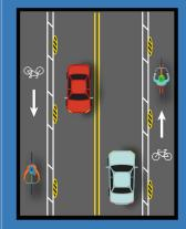
Protected bike lanes include bike lanes by the curbs, with buffer areas on the driving lane sides. The buffers include vertical devices that keep people driving from entering the bike lanes.
