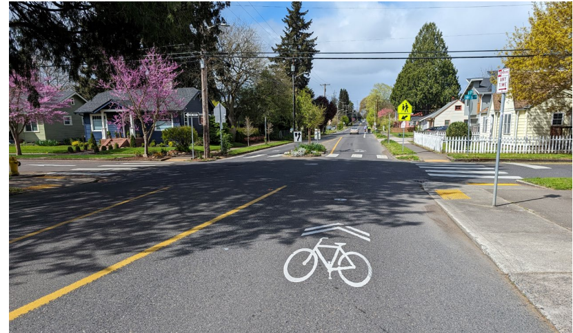
Figure 4: At midblock crossing locations east of N Street, the mobility lane changes to shared lane markings (sharrows), creating an inconsistent facility for bikes and small mobility.
